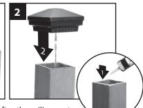
**NOTE:** Install post cap lights after the railing system post sleeve skirt, and post sleeve have been installed.
