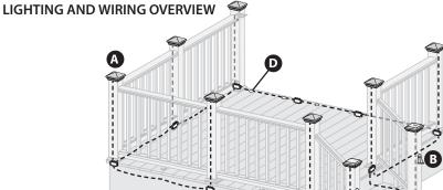
NOTE: All wiring and splitters are mounted to inside of framing, picture is just representation of where to place these in general
