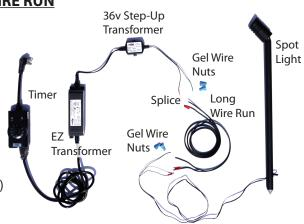
NOTE: One 36v Step-Up Transformer will support up tp 5 Spot Lights which is the same amount that can be connected into the Outdoor Splitter. There is a slight voltage drop on the 36v Step-Up Transformer as additional lights are added to the circuit resulting in a slight loss of light output.
