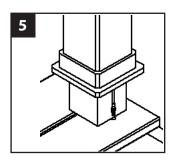
8. Place the bracket against the post with the wire hole lined up to the hole drilled in the post. Secure the bracket down with #6 wood screws or #6 self tapping screws for an aluminum post.
