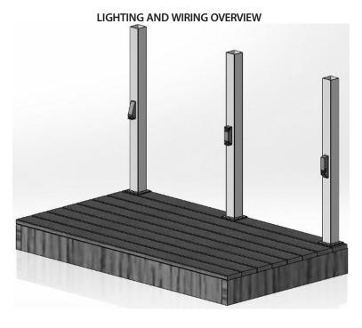
**NOTE:** All wiring and splitters are mounted to inside of framing, picture is just representation of where to place these in general.
