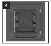
5. The post cap is designed for a wedge fit over the metal post. Add silicone buttons to the wedge faces of additional means of securing the post cap.
