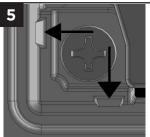
6. Set the post cap on the metal post. Then press down on the angled faces so the internal wedge tabs make a snug fit. Caution: Do not press down on the solar panel face.
