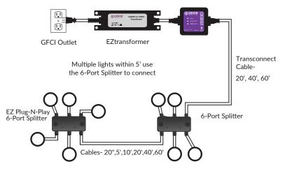
EZ Plug-N-Play 6-Port Splitter, T-Splitters, and Female-to-Female connectors can be used interchangeably depending on the needs of the location.
